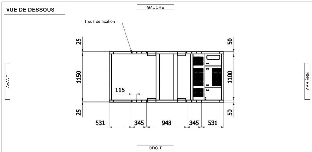
**DIMENSIONS AVEC PORTES OUVERTES (mm)**
