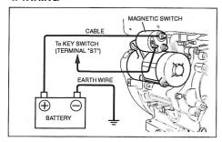
Connect positive (+) terminal of the magnetic switch and positive (+) terminal of the battery with battery cable.
