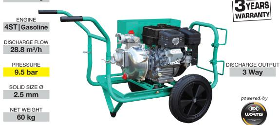
Our high-pressure construction pumps effectively move water over long distances or to great heights. They feature large-diameter impellers with shallow vanes for greater pressures and discharge heights, which allows the pumps to move water farther. They are ideal for sprinklers, moving water uphill, handling fast seepage or light firefighting while waiting for emergency crews to arrive.
