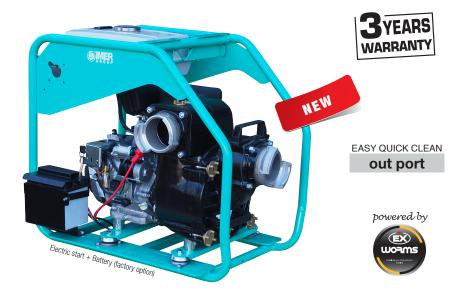
Built around durability, our SWT gasoline trash pumps feature a silicon carbide seal and a unique conical cast iron impeller design and a quickclean out port for easy maintenance and long service life. They reduce wear from abrasive materials and can handle solid objects up to 31 mm in diameter. There's even a strainer to ensure nothing bigger gets through.
