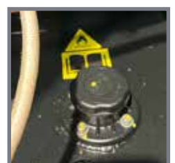
FUEL FILLER CAP Securely located inside to prevent theft
