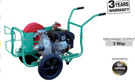
Our high-pressure construction pumps effectively move water over long distances or to great heights. They feature large-diameter impellers with shallow vanes for greater pressures and discharge heights, which allows the pumps to move water farther. They are ideal for sprinklers, moving water uphill, handling fast seepage or light firefighting while waiting for emergency crews to arrive.
