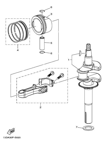
FIG. 2 CRANKSHAFT & PISTON
